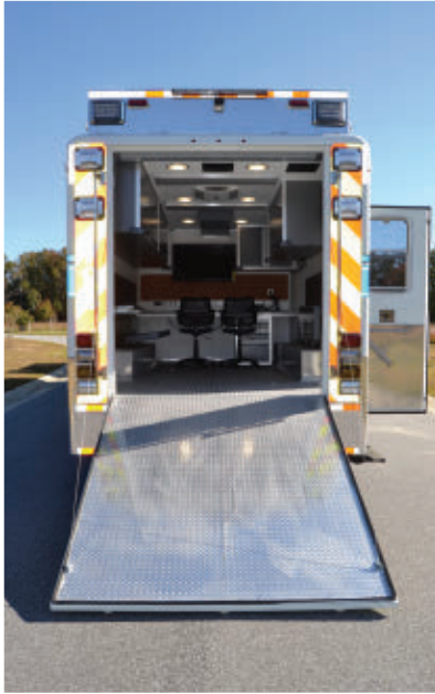
The rear of the trailer with a ramp for a robot and an area for the command center.
