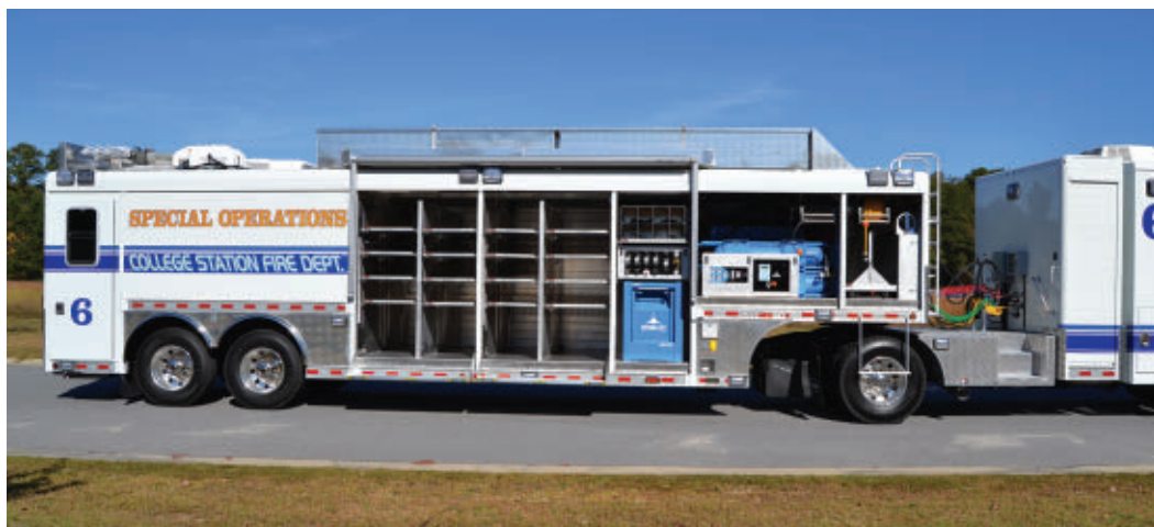
The trailer has large compartments and houses an air compressor and cascade system.
